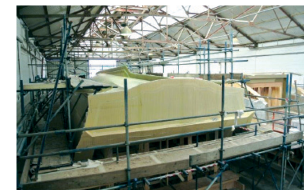
Epoxy infusion for Solution60, a 60ft power boat
