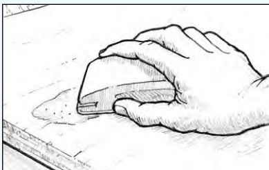
Figure 23 Sand cured fairing compound to desired contour.
