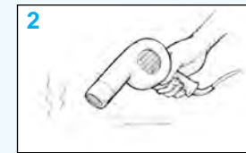
Figure 7 Dry the Surface. Allow wet surfaces to dry thoroughly or use heat or a fan to speed the drying.
