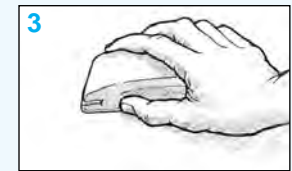
Figure 8 Sand non-porous surfaces. Provide a texture for the epoxy to key into.
