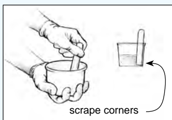
Figure 3 Stir resin and hardener thoroughly together for 2 minutes, longer in cooler temperatures.
