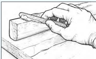
Figure 10 Apply thickened epoxy to one of the bonding surfaces.
