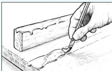
Figure 9 Apply resin/hardener mixture to the bonding surfaces.
